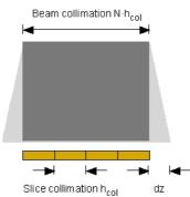
**Fig. 1** Dose profile free-in-air for a quad-slice scanner (dark grey: umbra, light grey: penumbra); overbeaming is characterized by the parameter dz.
