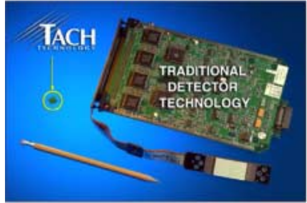
Fig. 3.14 The spatial requirements of an increased number of detector rows and the exorbitantly increased data rate necessitated the development of data acquisition systems with tiny application-specific integrated circuits (ASIC’s) that replaced the traditional circuit boards (courtesy: Philips Medical Systems).
