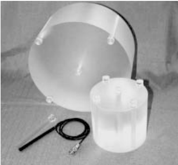
Fig. 3.4 Cylindrical standard CT dosimetry phantoms (16 and 32 cm in diameter) made from Perspex for representative measurements of CTDI in regions of the head and the trunk and a pencil-like detector for measurements of the dose profile integral.
